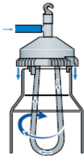
Fig. 1.19 An in-can cooler is placed on top of the milking bucket or any type of milk can.
